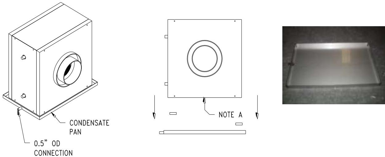
***NOTE A: Drill a 3/8" hole carefully through the middle of the bottom to allow better free flow of water out of the coils sheet metal case.***
