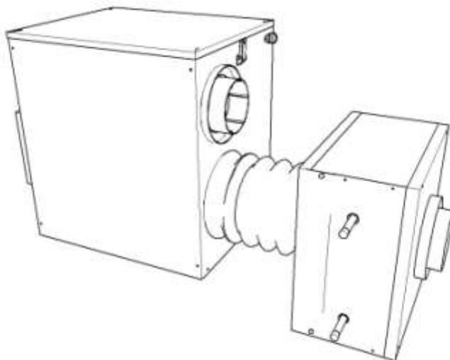
Connect to Duct 2 "Fresh Air In to the living space" noted on the RecoupAerator. Make this connection using insulated ducting. Be sure the air flow direction is consistent between the air stream, and the diagram. Screws, mastic, and/or metal tape are required after making the connection. It is important to have no air leakage.
