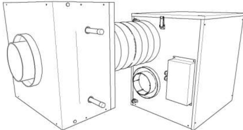
Connect to Duct 1 "Fresh Air In from outside" noted on the RecoupAerator. Be sure the air flow direction is consistent between the air stream, and the diagram. Screws, mastic, and/or metal tape are required after making the connection. It is important to have no air leakage. To prevent condensation from forming on the duct work, the duct must be insulated and air tight from the outside wall to the duct connection of RecoupAerator. The coil case is insulated.
